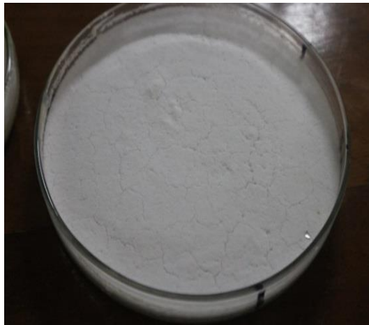
Picture 1. Polyethylene microplastic from the dried scrub soap
